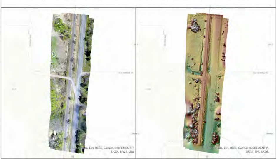
442nd St, Harris, MN – 082750K Orthophoto and hillshaded DEM results from 200ft (61.0m) sight line flights
