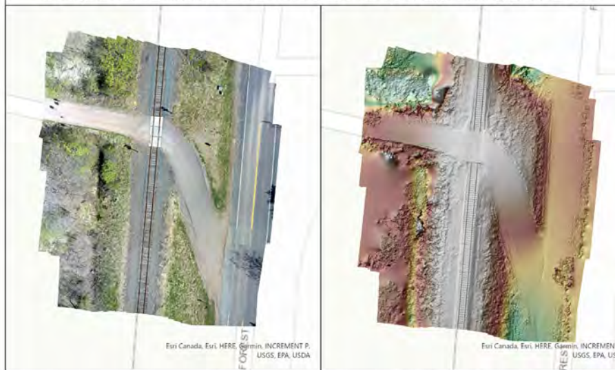
442nd St, Harris, MN – 082750K Orthophoto and hillshaded DEM results from 80ft (24.4m) crossing profile flights
