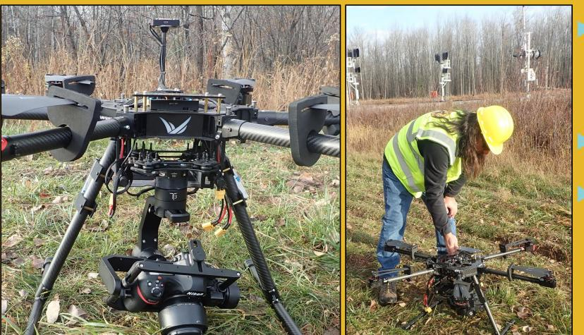
Crossing-i uses a single customized drone platform (Tarot X6) capable of autonomously performing a pre-planned flight mission
